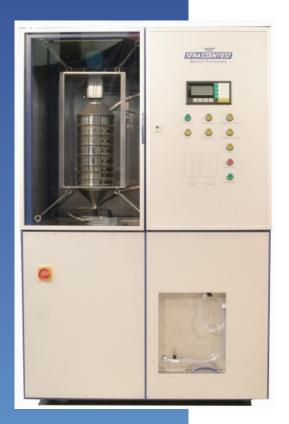
The new Automatic Binder Extraction Machine according to the cold extraction process DIN 1996, part 6, works almost emission-free which meets the requirements of personal and environment protection.
