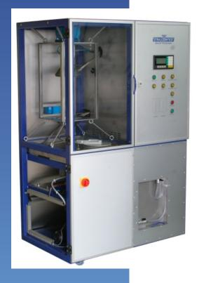
Function and application of this system is identical with our Automatic Extraction Machines type 419/518, catalogue no. A00131, for non-inflammable solvents which serves best results in asphalt laboratories since more than 20 years.
