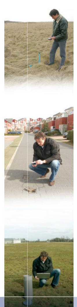
The **CTD-Diver** is a compact instrument that allows you to measure the ground water level, ground water temperature and conductivity of the ground water all in one. Where monitoring ground water, especially where it concerns decontamination of polluted soil, the monitoring of rubbish dumps and the detection of salination, once used to be a labour-intensive and troublesome job, the arrival of the CTD-Diver has changed all that.
